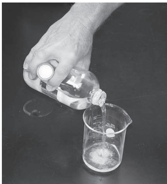
Figure 1-11. Holding a reagent cap while pouring reagent.
